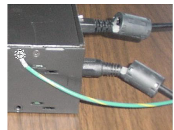
This partial view of the data acquisition device shows its connection to the ground-line. It also shows two ferrite collars, the foremost of which is clamped to the power cable. The background collar is clamped onto the Ethernet cable.
